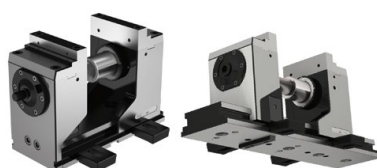
Alignment through 20 H7 precision slot nuts in the base body (H5G) and alignment sets 14 / 16 / 18 in the machine table's T-slot. Clamping with clamping claws.
