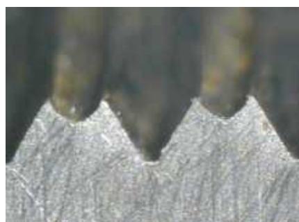
Underformed – core hole too large
