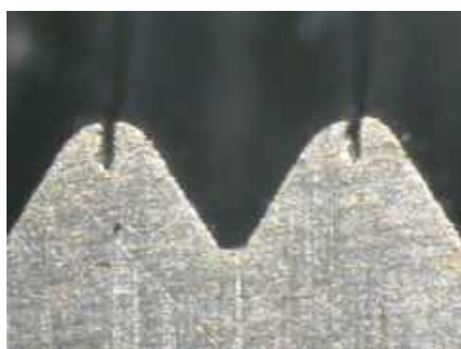
Overformed – core hole too small
