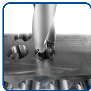
Vollbohren Solid drilling
