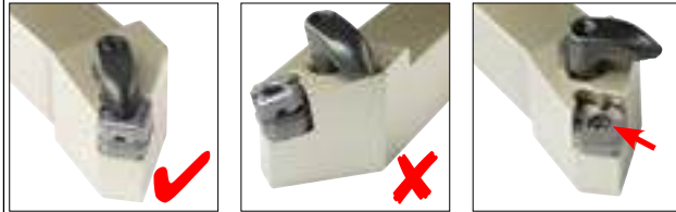
Correct insert position
