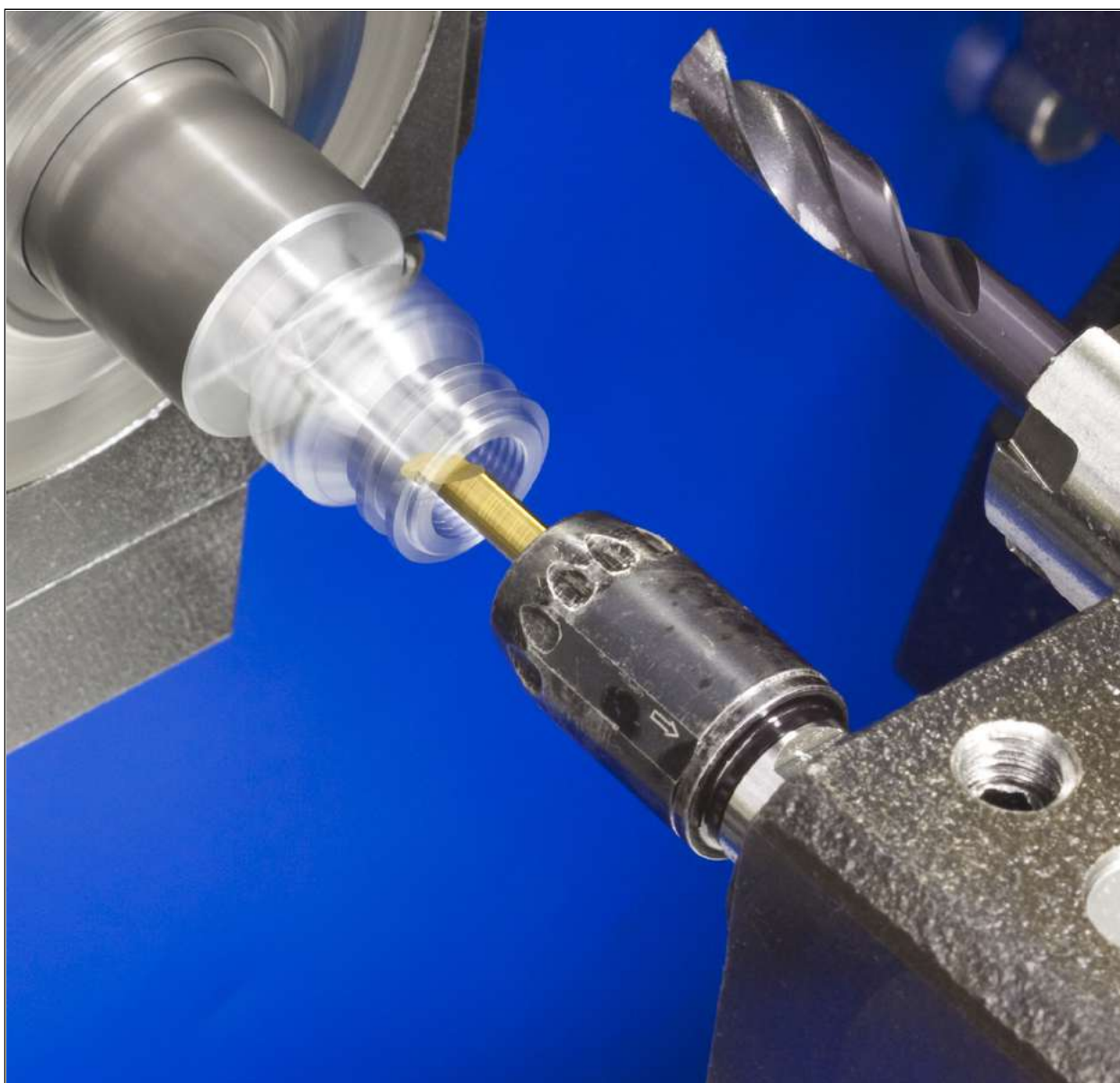
GHPCOR perpendicular square-shank tools for use on cross slide units of swiss-type and automatic machines
