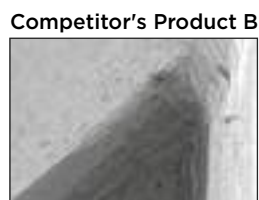
Chipping in edge coating
