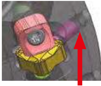
Multi-tooth design via wedge clamp (3.5 teeth/inch)
