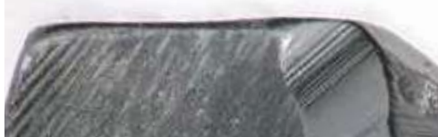
After drilling 900 holes
