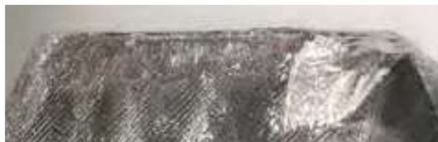
After drilling 3,840 holes
