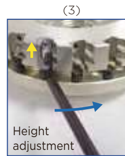
(3) Adjust the blade to the required height by using the dedicated wrench to turn the height adjustment screw.
