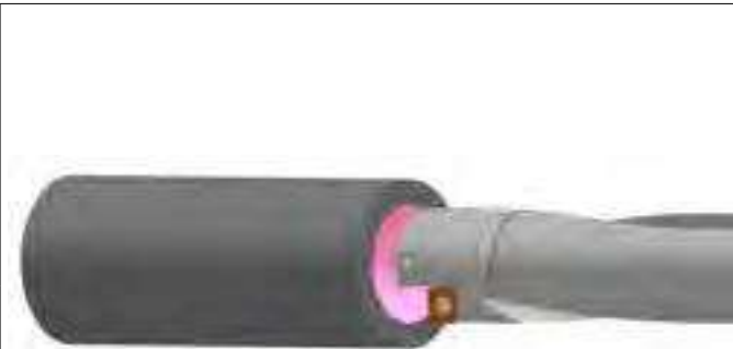
Deep hole drilling of H75mm from both ends
