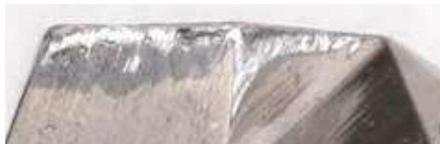
After drilling 900 holes
