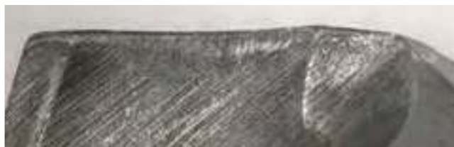
After drilling 3,840 holes
