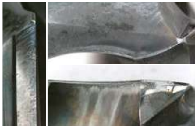
After drilling 2,500 workpieces (5 holes per workpiece)
