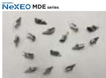
Chips are broken into small pieces
