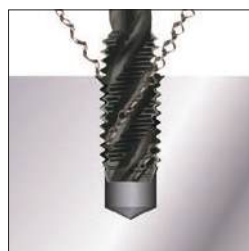
Chips from a tapped hole.
