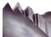
Close-up of VUSP after Tapping of 250 Holes
