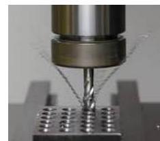
Chip evacuation with a SP tap.
