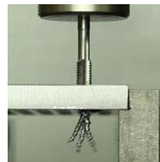
Chips discharge of a PO tap
