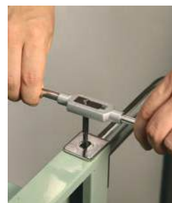
Hand tapping using a tap handle.
