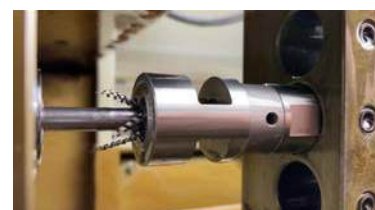
Chip evacuation status with DPO
