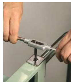
When hand tapping, always use tap wrench
