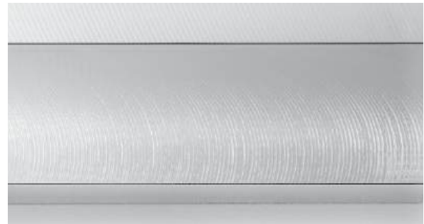
Surface Finish (Machining with Workpiece Overhang Length of 80mm)
