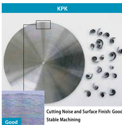
Cutting Performance Comparison (Internal Evaluation)
