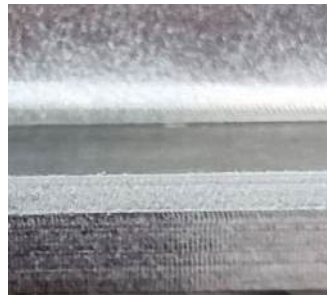
Material C45 machined with 208181.
