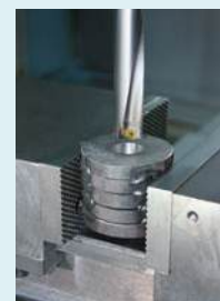
Drilling through stacked components.
