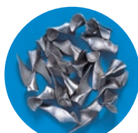
SUS304 EX-SUS-GDR \phi 8.5 Speed: 18m/min Feed: 0.2mm /rev
