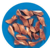
C1020(Copper) EX-SUS-GDR \phi 8.5 Speed: 32m/min Feed: 0.24mm /rev
