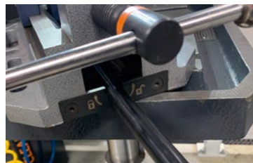
Open and lock the clamping using the supplied clamp wrench.
