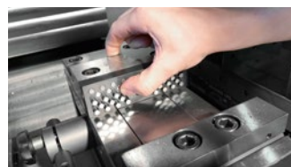
Positioning pins pushed in manually.
