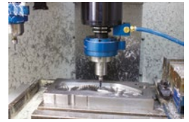
35 8825 Device for automatic tool changing on request.
