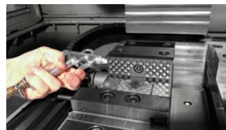
Actuation from both sides with a compressed air gun replaces the previous procedure of using the push-out pin with its obstructive contour.
