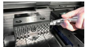
Actuation from both sides with a compressed air gun replaces the previous procedure of using the push-out pin with its obstructive contour.
