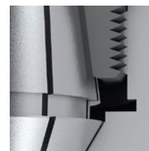
Standard ER chuck → Collets are not inserted 100% into the chuck.
