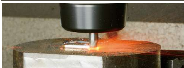
Machining HRSA by Ceramic Endmill
